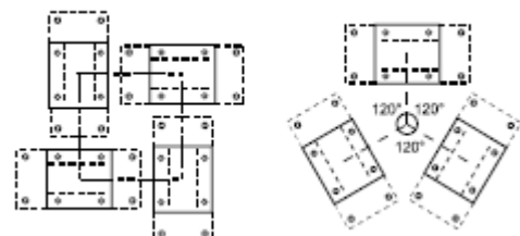
ORIENTATION OF WEIGH MODULES FOR 3-4 POINT SUPPORTS
