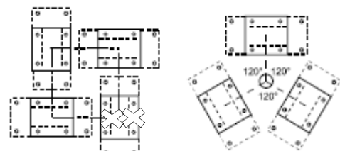
ORIENTATION OF WEIGH MODULES FOR 3-4 POINT SUPPORTS
